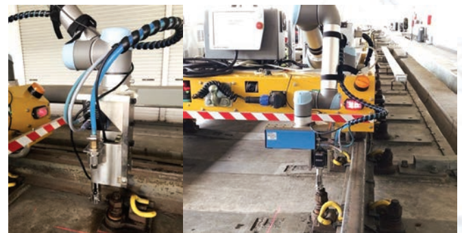
Figure 5: Unmanned Vehicle for Rail Fastening Bolt Inspection
